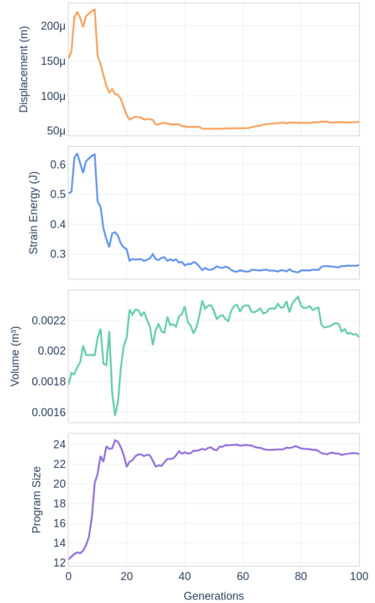
Fig. 3. Population means over generations for the three objectives (displacement in metres, strain energy in Joules, volume in cubic metres) and program size.
